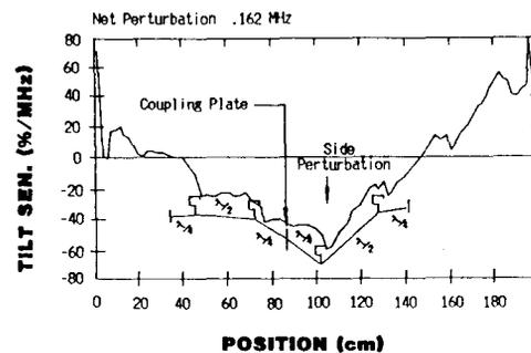
Fig. 6. Side-perturbation tilt of 0.3% coupling.
