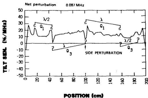
Fig. 4. Stabilized side-perturbation tilt sensitivity.
