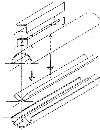
Fig. 1. Exploded view of RFQ with stabilizer.
