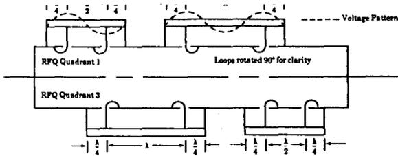
Fig. 2. Stabilizer schematic.
