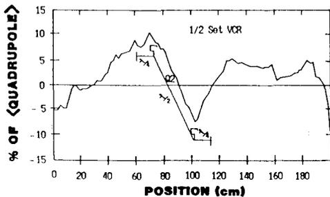
Fig. 8. Dipole mode component of RFQ (half set).
