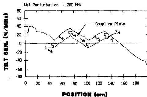
Fig. 5. End-to-end tilt of 0.3% coupling.
