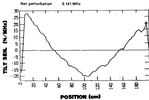
Fig. 3. Unstabilized side-perturbation tilt sensitivity.
