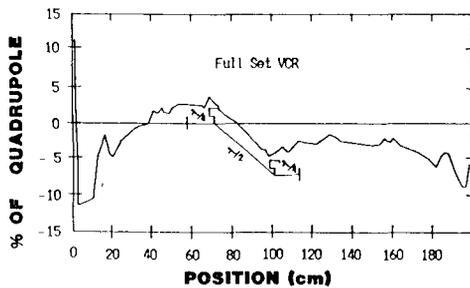
Fig. 7. Dipole mode component of RFQ (full set).
