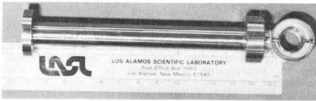
Fig. 2. The concentric inner and outer rings of capacitive probe #1 are connected to a 50- $\Omega$  back-termination resistor and a SMA coaxial connector.
