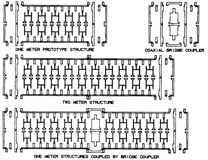
Fig. 2 Disk and Washer Linac configurations
