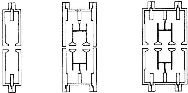
Fig. 3 One, two and three cell frequency test configurations
