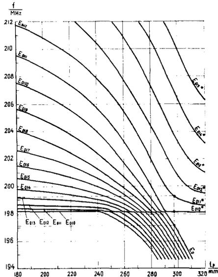
Fig. 2. Frequency spectrum transformation vs. the length of posts.
