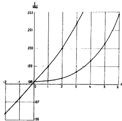
Fig. 5. Dispersion curve of cavity No.1 before (o o o) and after (• • •) stabilization.
