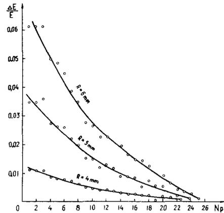
Fig. 1. Dependence of the systematic error due to a field nonuniformity in the gap at the various bead diameters.
