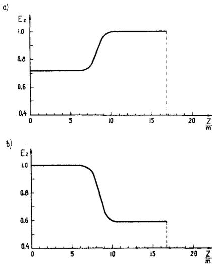
Fig. 3. The effect of tab rotation on the  $E_{010}$  field distribution:
