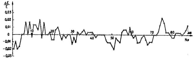
Fig. 4. The accelerating field distribution in cavity No.1 after tuning.
