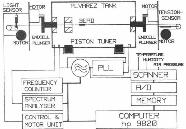
Fig. 1 Block diagram of the measurement set-up
