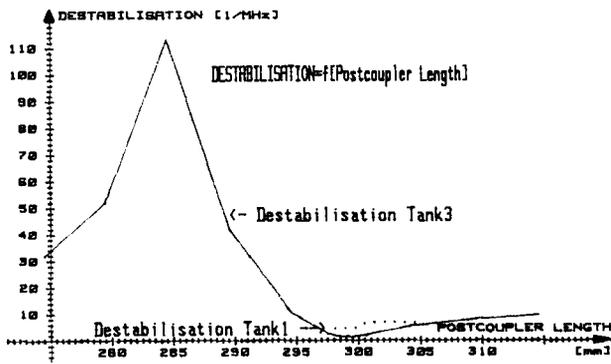
Fig. 4 Destabilisation as function of postcoupler length for tank 1 and tank 3
