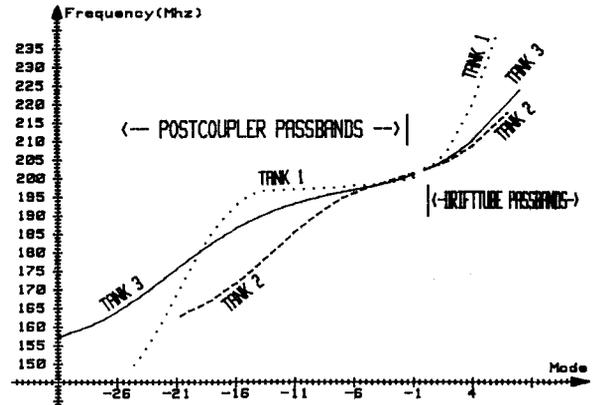
Fig. 3 Postcoupler and drifttube passbands
