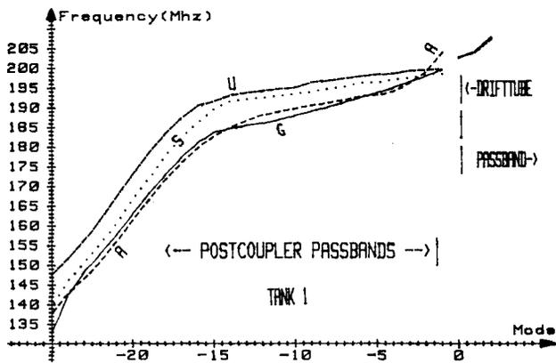
Fig. 5 Postcoupler passbands for different postcoupler settings which are shown in fig. 6
