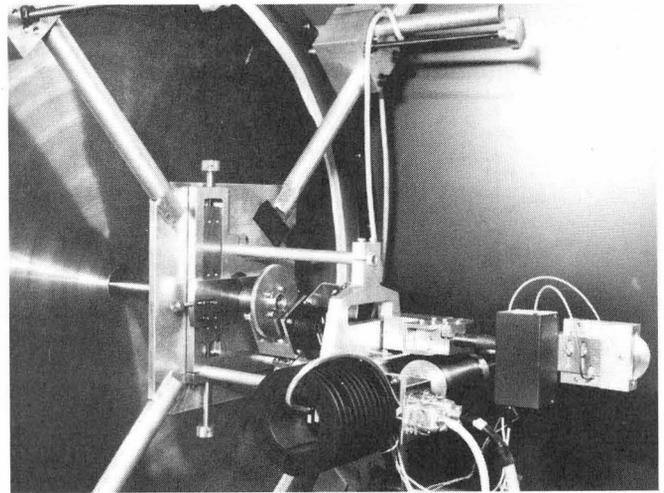
Fig. 2 Step motor unit with light sensor and endcell plunger
