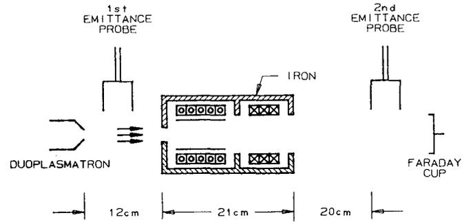
Figure 2: Experimental layout for Gabor lens Measurements
