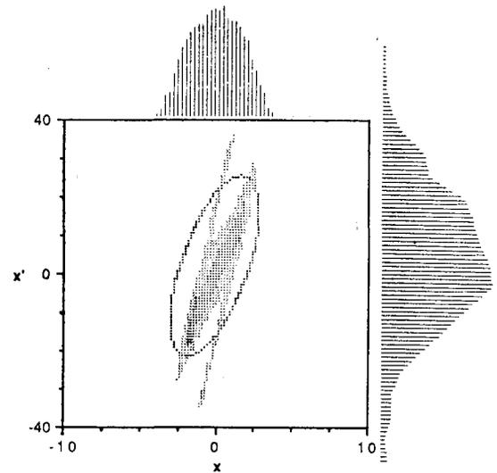
Figure 3: Source emittance;  $\alpha = -.77$ ,  $\beta = 0.15$ ,  $\epsilon_{rms} = .56$ ,  $\epsilon_{90\%} = 0.247$ ,  $I = 11$  mA. The projection of the distribution on the  $x$  and  $x'$  axes are shown. Units are mm and mrad. The rms ellipse is shown.
