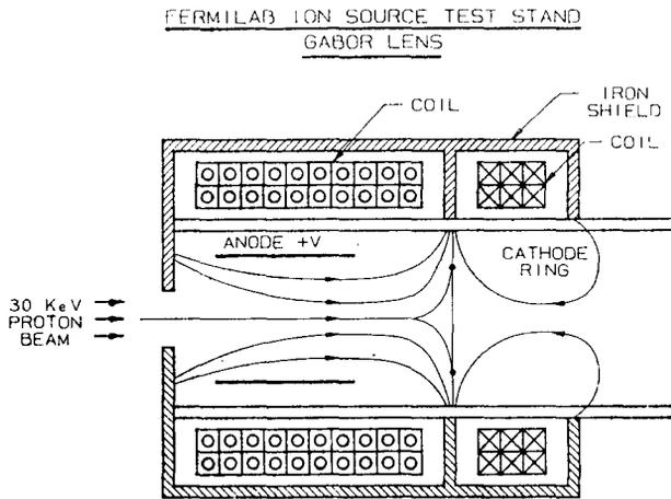
Figure 1: Gabor lens with cusped magnetic field
