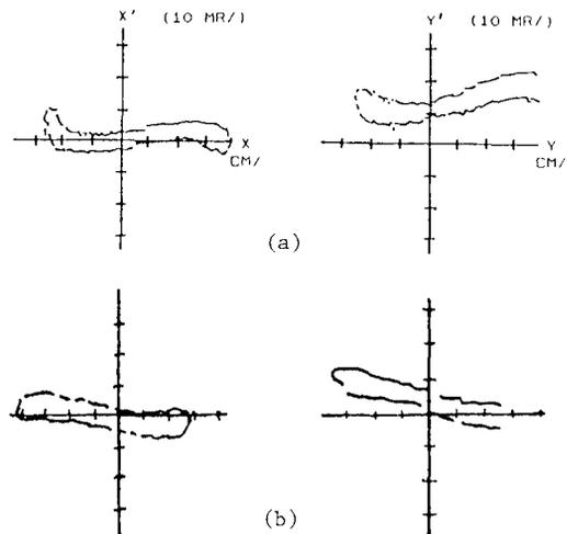
Fig. 2. Emittances measured at E1 in the 35 keV line for (a)  $\phi_{\text{anode}} = 2$  mm, electrode gap = 3 mm (CASE 1),  $E_n(90\%) = 0.11 \pi$  cm-mrad; (b)  $\phi = 2.8$  mm, gap = 3.5 mm (CASE 2),  $E_n(90\%) = 0.11 \pi$  cm-mrad (CASE 2); (c)  $\phi = 2.8$  mm, gap = 4 mm (CASE 3--not shown).
