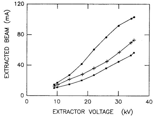
Fig. 5. Current extracted from magnetron, measured at X1, vs extractor voltage. ● = Case 1; + = Case 2; ■ = Case 3.
