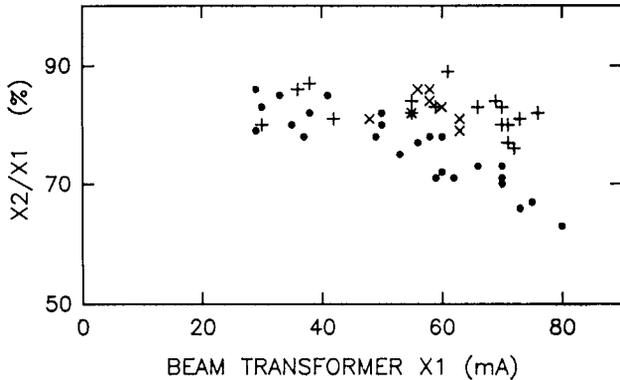
Fig. 3. Transmission through the RFQ vs beam current measured at X1: ● ≡ Case 1; + ≡ Case 2; x ≡ Case 3.
