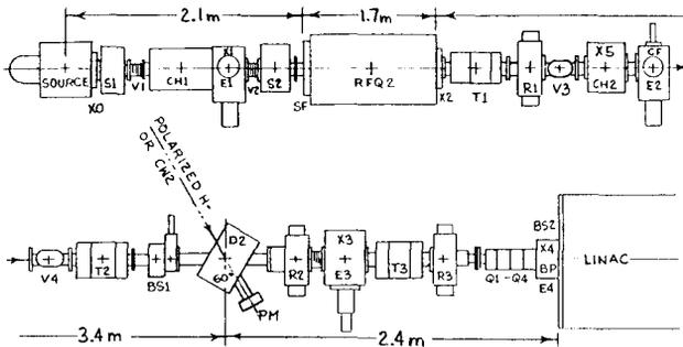
Fig. 1. Layout of the new RFQ preinjector beamline: BP-Beam phase probe; BS-Beam stop; CF-Coaxial Faraday cup; CH-Chopper; D2-Bending magnet; E-Emittance analyzer; Q-Quadrupole; R-RF cavity; S-Solenoid lens; SF-Segmented Faraday cup; T-Quadrupole triplet; V-Vernier steering magnet; X-Beam current transformer; PM-Profile monitor.
