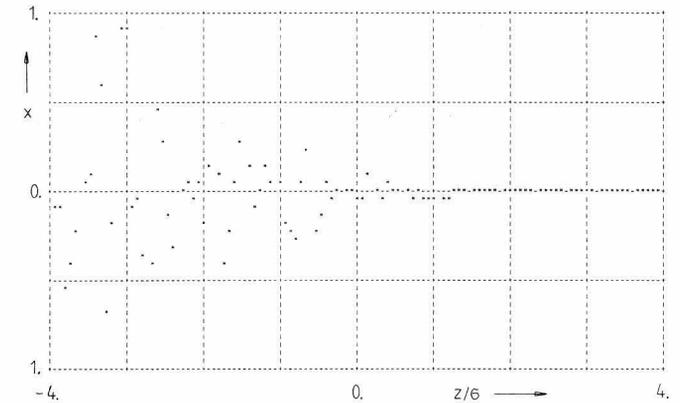
Fig. 4 Bunch shape in the case of random RF structure displacement, unit r.m.s. value, and on-axis injection (at the end of the CLIC linac).
