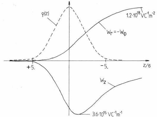
Fig. 1 Wake fields of the CLIC RF structure.
