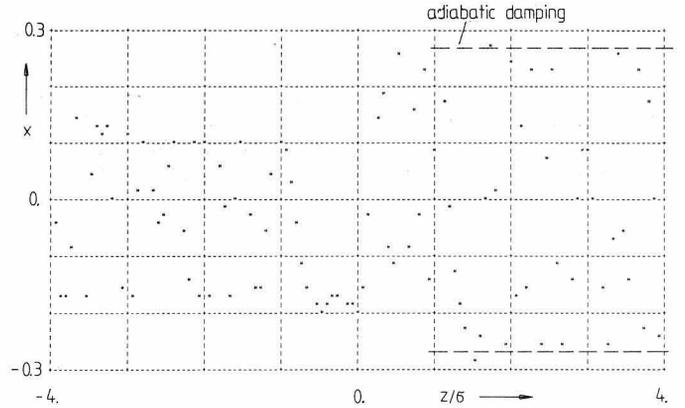
Fig. 3 Bunch shape in the case of real energy spread, a perfectly aligned machine, and unit value injection offset (at the end of the CLIC linac).
