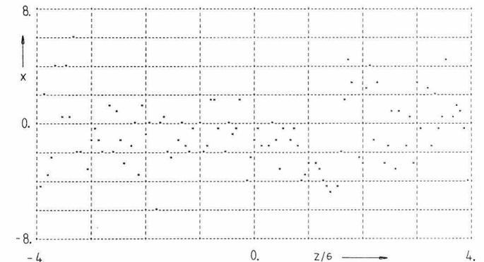
Fig. 5 Bunch shape in the case of random quadrupole displacement, unit r.m.s. value, and on-axis injection (at the end of the CLIC linac).
