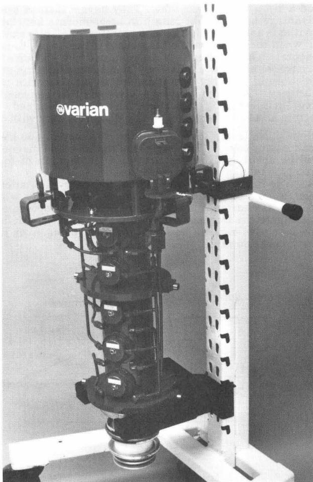
Fig. 3. Varian VKP7990 klystron with depressed collector.
