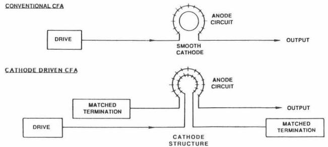
Fig. 4. CFA schematic showing a conventional CFA and a cathode-driven CFA.
