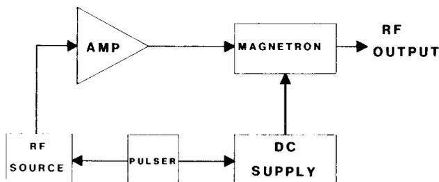
Fig. 6. Phase-locked magnetron block diagram.
