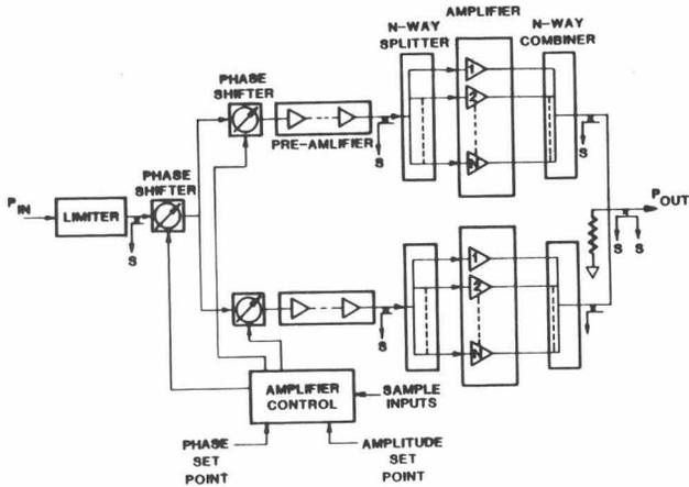
Fig. 12. Solid-state amplifier block diagram.
