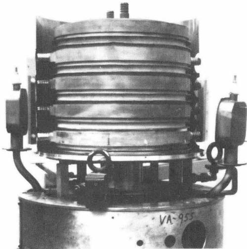
Fig. 2. Depressed-collector construction.
