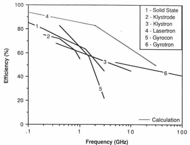
Fig. 11. (Efficiency vs frequency for various rf power devices.
