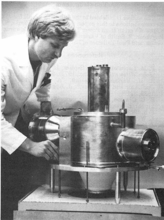
Fig. 9. Klystron ready for test.
