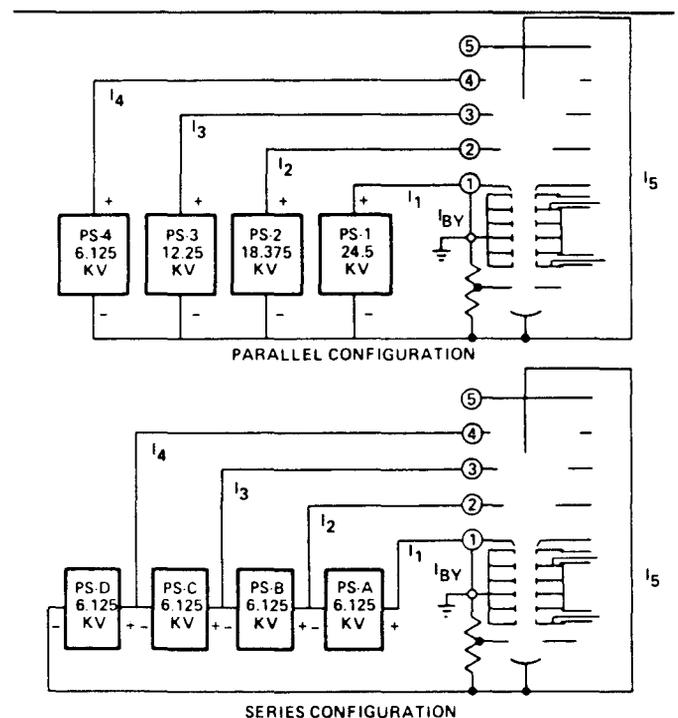
Fig. 1. Multistage depressed-collector schematic.
