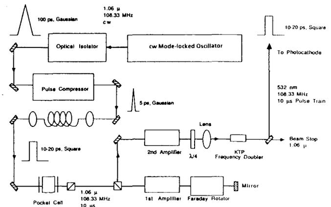
Fig. 2. Block diagram of the photocathode illuminator consisting of a cw mode-locked Nd:YAG oscillator and pulsed amplifiers.
