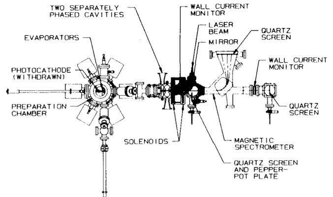
Fig. 1. Photoinjector, two-cavity experiment.
