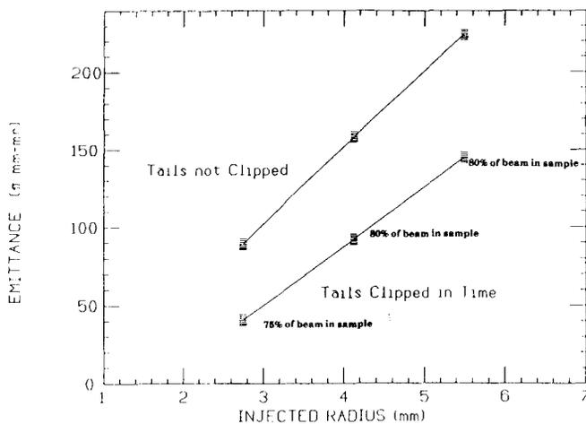
Fig. 4. Emittance vs injected pulse radius.
