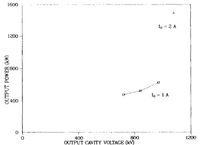
Fig. 2. Calculated output power versus output cavity voltage for the system of Fig. 1, with average beam current as the parameter.
