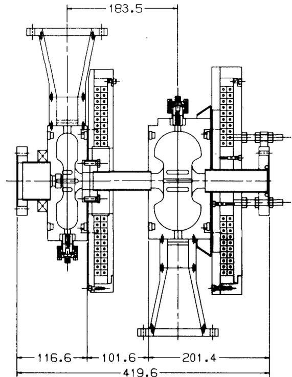
Fig. 5. Scale drawing of the rf-driven lasertron (dimensions in millimeters).
