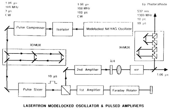
Fig. 4. Block diagram of the mode-locked laser system.
