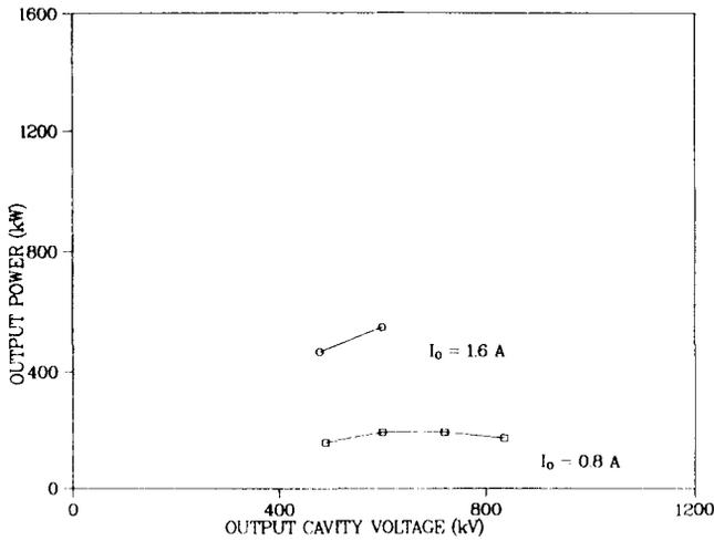
Fig. 3. Calculated output power versus output cavity voltage for the five times lasertron frequency multiplier, with average beam current as the parameter.
