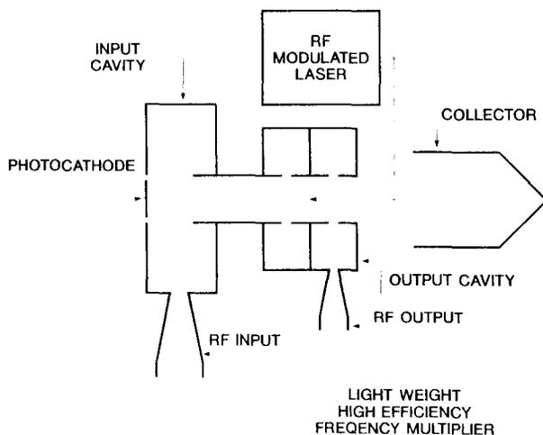
Fig. 1. Schematic drawing of the rf-driven lasertron experiment.
