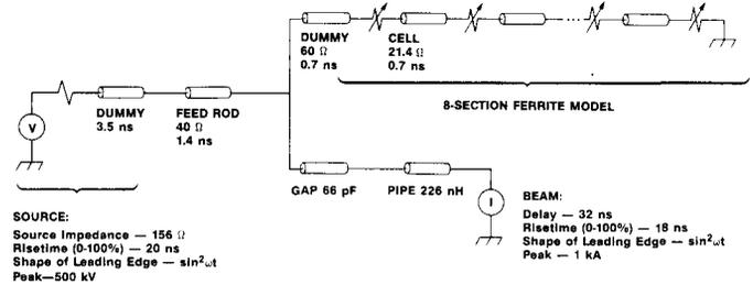
**Figure 7.** Equivalent circuit for proposed LIA cell. Nonlinear resistor characteristics defined as described in text. Dummy transmission line elements inserted to satisfy circuit topology constraints of circuit analysis code.
