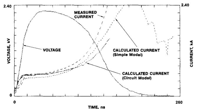
**Figure 4.** V-I characteristics and calculated current from both the simple ferrite model and circuit model for core tested in Shot W193. Circuit model assumes axial displacement currents with  $\epsilon = 12$ . Core dimensions listed in Table 1.  $\alpha = 0.5$ .
