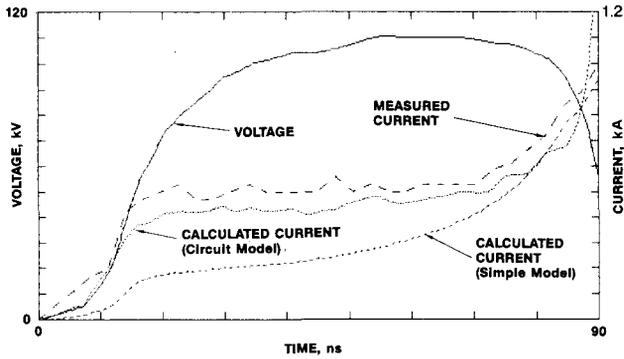
**Figure 5.** V-I characteristics and calculated current from both the simple ferrite and circuit model for ETA-II cell taken from References 2 and 3. Circuit model assumes radial displacement currents with  $\epsilon = 12$ . Ferrite dimensions listed in Table 1.  $\alpha = 0.5$ .
