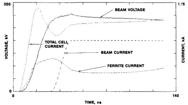
**Figure 8.** Calculated response of proposed LIA cell obtained with the circuit model as shown in Figure 7. Ferrite dimensions listed in Table 1. Radial displacement current flow and  $\alpha = 0.5$  assumed.
