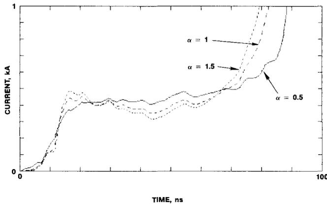
**Figure 6.** Calculated current from the circuit model for ETA-II cell for three values of  $\alpha$ .
