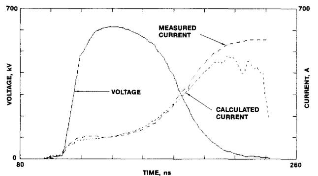
**Figure 3.** V-I characteristics and calculated current from simple ferrite model for core tested in Shot W157. Core dimensions listed in Table 1.  $\alpha = 0.5$ .
