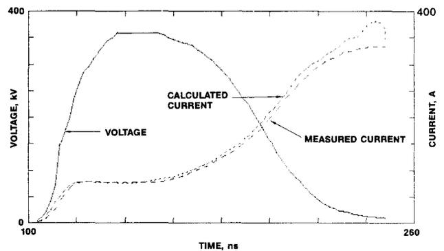
**Figure 2.** V-I characteristics and calculated current from simple ferrite model for core tested in Shot W163. Core dimensions listed in Table 1.  $\alpha = 0.5$ .
