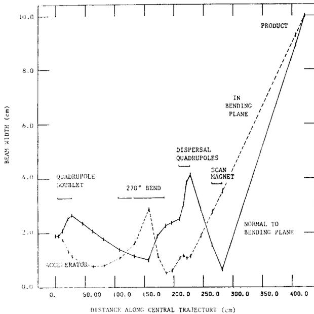
Fig. 3 Beam width along the 270° bend spot-scan beam delivery system.
