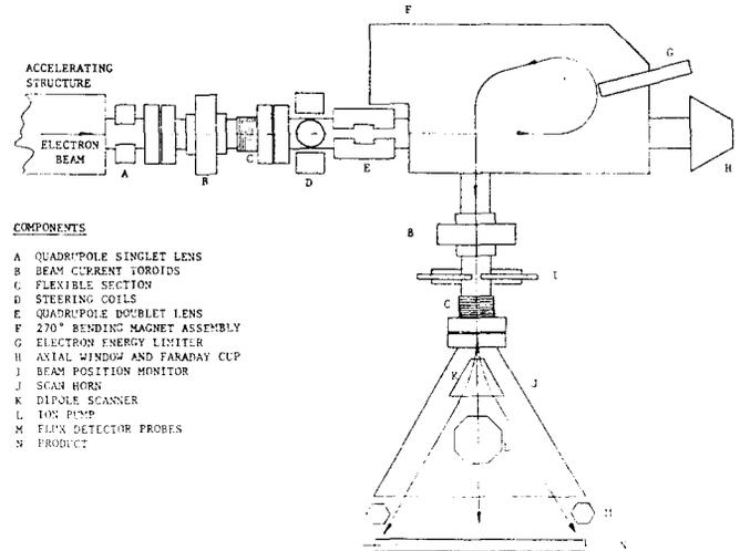
Fig. 1 I-10/1 beam delivery system.
