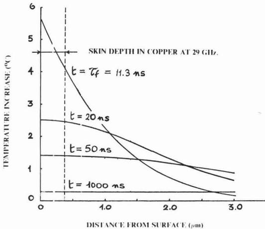
Fig.2 Temperature increase in the surface layer.
