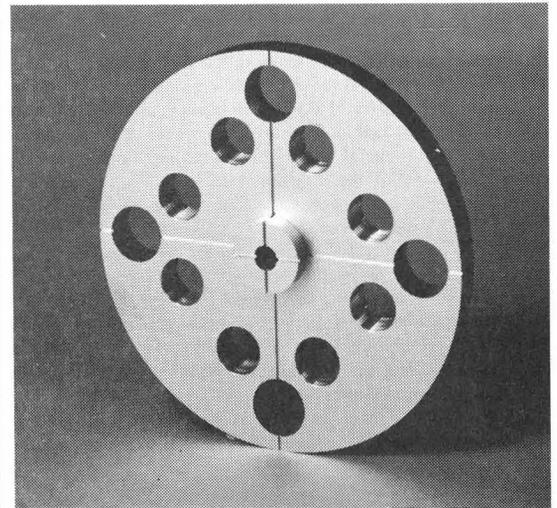
Fig.9 Cut through CLIC cross section showing transverse slots.
