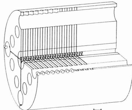
Fig.4 Conceptual design of the CLIC accelerating structure.
