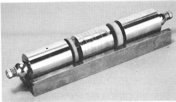
Fig.7 Alignment in V-block prior to brazing.
