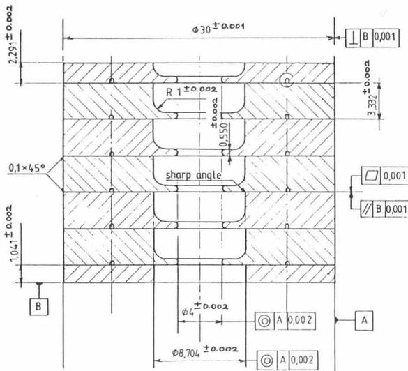
Fig.6 Short test stack of precision machined cups (29.985 GHz).
