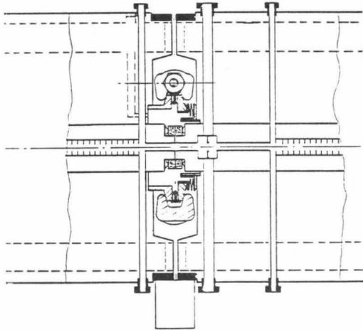
Fig.5 Connection between CLIC modules.
