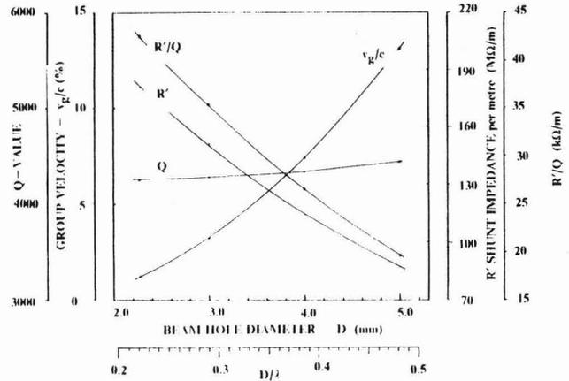
Fig.1 Variation of structure parameters with beam hole diameter.
