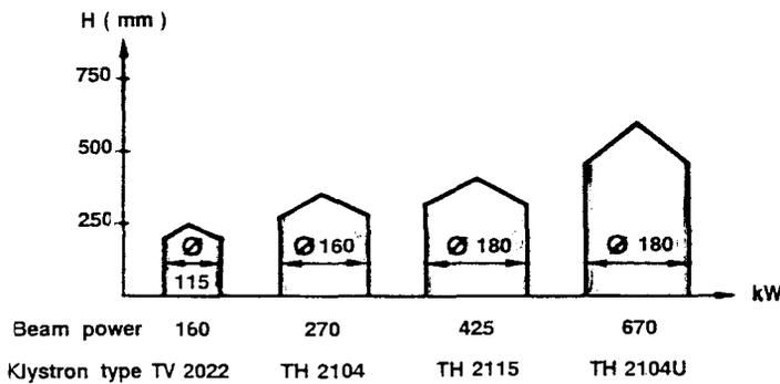
Figure 3 - L-band klystron collectors
