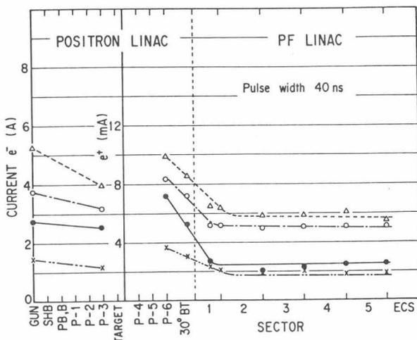
Fig. 6 Beam currents along the accelerator for 40ns pulse
