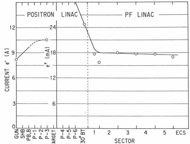
Fig. 4 Beam current along the accelerator, may, 1988
