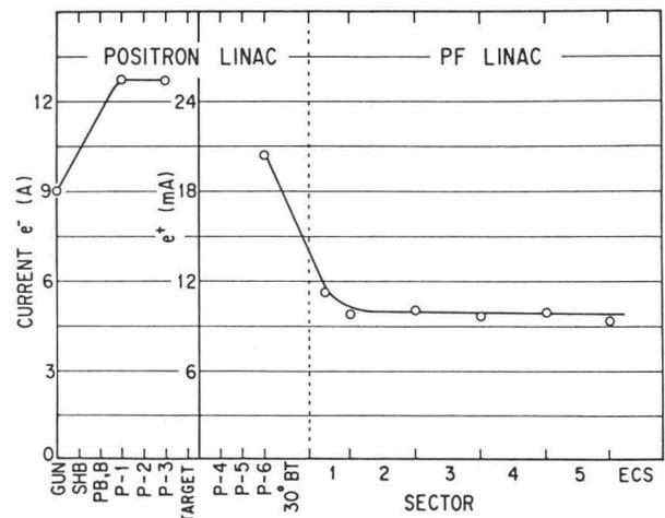
Fig. 2 Beam current along the accelerators , Nov., 1987.
