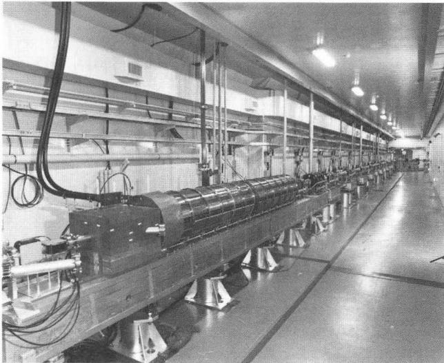
Fig. 1 Positron producing target and positron accelerator of the generator.
