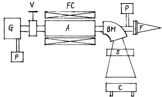
Fig.1 Schematic diagram of radiation processing linac
