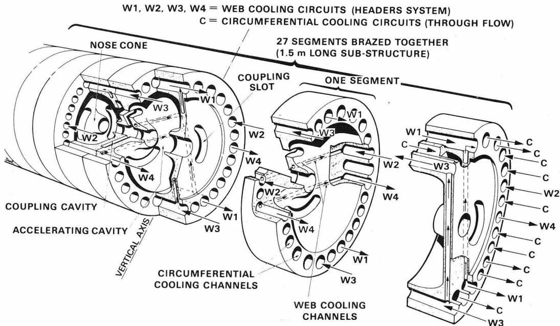
Fig. 3 Cooling circuits of the 1300 MHz on-axis coupled structure.
