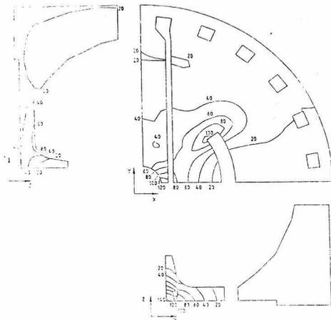
Fig. 4 Von Mises stress contours in the cavity walls at a power level of 150 kW/m (stresses in MPa).
