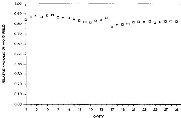
Fig. 6 Average on-axis electric field distribution in the IMPELA prototype cavities.
