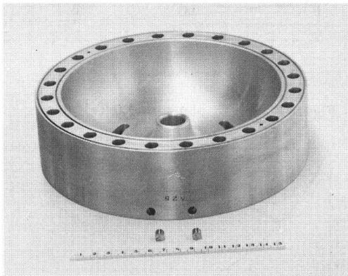
Fig. 1 IMPELA basic cavity segment.
