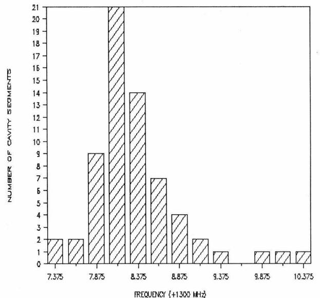
Fig. 5 Histogram of the accelerating half-cavity frequency after machining with a numerically controlled lathe.
