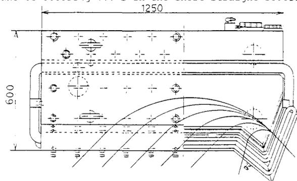
Fig. 2. Layout of the sector magnet EM4. EM1 has the same dimension in mirror symmetry.
