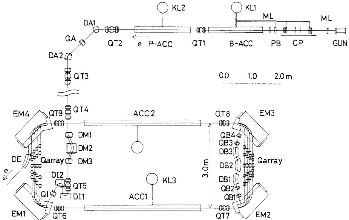
Fig. 1. Layout of the 35 MeV CW double sided microtron and the 5 MeV injector. KL:klystron, ML:magnetic lens, CP:chopper, PB:prebuncher, B-ACC:buncher, P-ACC:pre-accelerator, DA and QA:analyser magnets, DM:longitudinal matching magnet, DI and QI:injection magnets, EM:sector magnet, ACC:4m tube, DB and QB:phase matching magnets, DE:extraction magnet, QT:Q-tripet.
