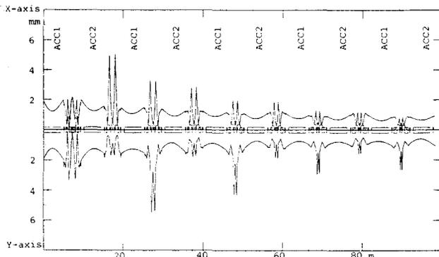
Fig. 5. First order calculation of envelopes from entrance to the first ACC1 to exit of the fifth ACC2.
