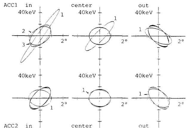
Fig. 6. Behavior of longitudinal beam ellipse during acceleration in the DSM when injected with matched condition. The number of recirculation is indicated.
