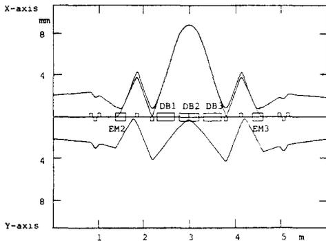
Fig. 3. Envelopes in the phase matching system.
