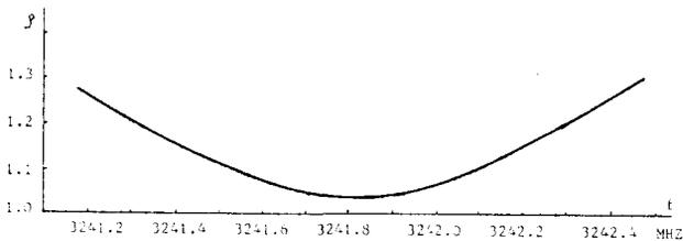
Fig.4  $\rho \sim f$  curve of TW DAW Tank
