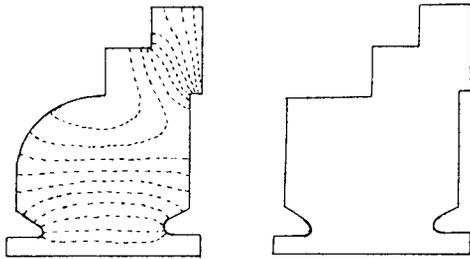
Fig.1 field distribution of the coupler for TW DAW Fig.2 coupler structure made actually.
