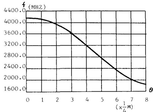
Fig.5 Dispersion curve of the DAW structure
