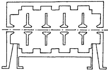
Fig.3 The established TW DAW Tank
