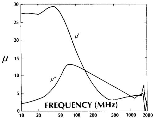
Figure 1. Relative Permeability ( $\mu'$ ) and Loss Tangent ( $\mu''$ ) vs Frequency
