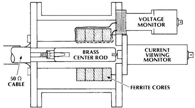
Figure 2. 20 kV Ferrite Core Testing Fixture
