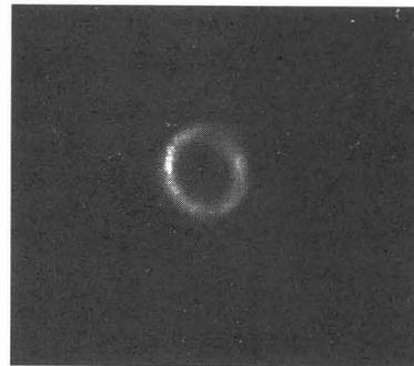
Fig. 9. Time-integrated pinhole photograph of the beam from the new injector. The slight ellipticity is due to a small parallax between the beam and camera axis.
