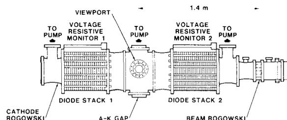
Fig. 1. RADLAC-II injector cavity.
