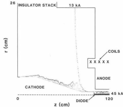
Fig. 7. Electron map for the new injector. The applied voltage to the A-K gap is 4.75 MV. All the electron losses occur radially and account only for 13 kA of the 58 kA total shank current.
