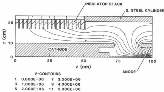
Fig. 2. Equipotential plot for the old cathode field shaper. The anode voltage is 5 MV.
