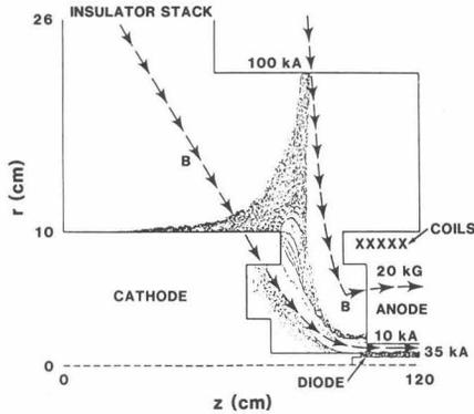
Fig. 3. Particle code simulation for the old injector geometry. The cathode shank current losses are 110 kA. The beam current is only 35 kA. The voltage is 5 MV. The arrows indicate two magnetic field flux lines.
