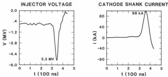
Fig. 4. Measured injector voltage and cathode shank current with the old injector.
