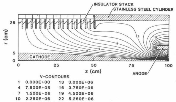
Fig. 6. Equipotential plot for the new conical field shaper.
