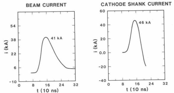
Fig. 8. Total shank and beam current for a 4.1 MV injector voltage. The shank current losses (=shank current minus beam current) are less than 11%.
