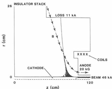
Fig. 5. Particle code simulation of the injector with a thin 2-cm diameter cylindrical cathode field shaper and shank. The voltage applied to the A-K gap of the diode is 4 MV. The total cathode shank current is 57 kA. The beam current is 46 kA.
