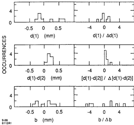
FIG. 3. Quadrupole misalignments  $d$  and BPM biases  $b$  calculated for eight quadrupoles in the overlap region between two overlapping sets, (1) and (2), of 16 quadrupoles each. The data plotted are from the vertical plane of SLC Linac Sector 2.
