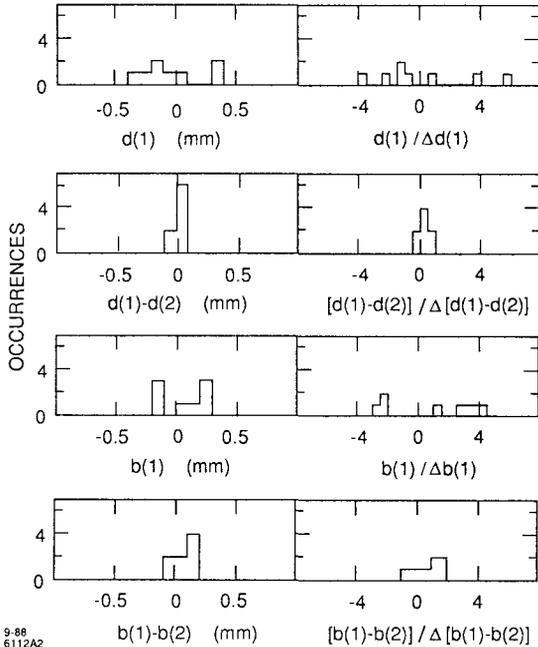
FIG. 4. Quadrupole misalignments  $d$  and BPM biases  $b$  calculated from two different two-beam trajectories, (1) and (2), through the same eight quadrupoles in the vertical plane of SLC Linac Sector 2.
