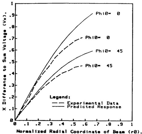
Figure 3 X axis difference-to-sum voltages versus position normalized to beampipe radius  $a$ .
