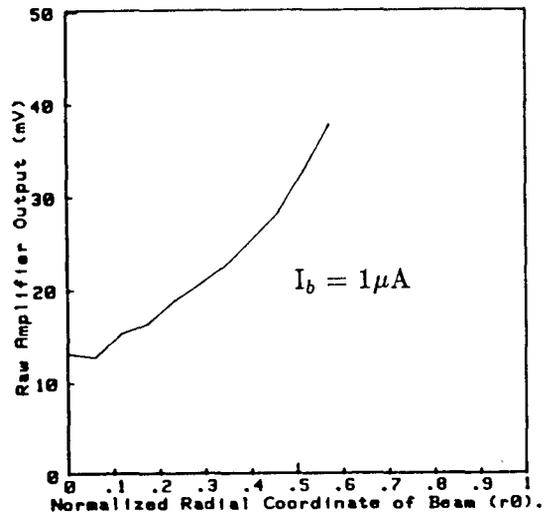
Figure 2 Voltage output of a single channel versus beam position normalized to beampipe radius  $a$ .
