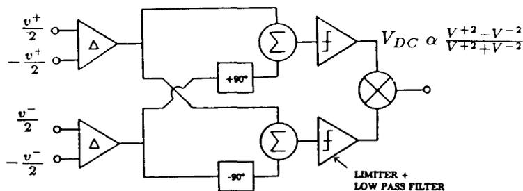
Figure 5 Amplitude-to-phase converter/detector.
