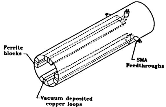
Figure 4 Concept for final pickup design.
