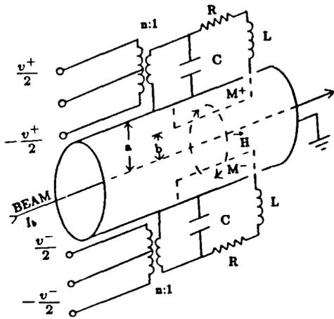
Figure 1 Schematic illustration of inductive loop pickups.
