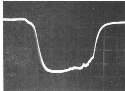
Fig.5.  $\text{H}^-$ -injector exit beam current. The vertical - 5 mA/div, the horizontal -  $20\mu\text{s}/\text{div}$ .
