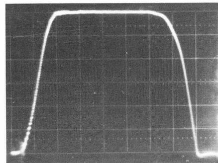
Fig.2. Accelerating voltage pulse. The vertical - 125 kV/div, the horizontal -  $20 \mu\text{s}/\text{div}$ .
