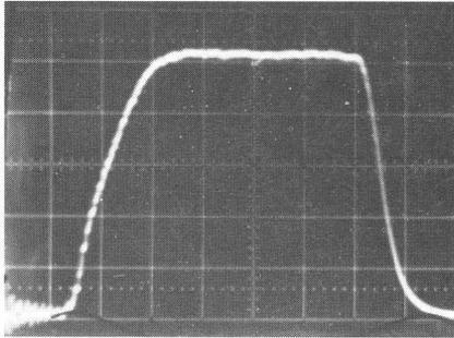
Fig.3. Proton injector exit beam current. The vertical - 40 mA/div, the horizontal -  $20\mu\text{s}/\text{div}$ .
