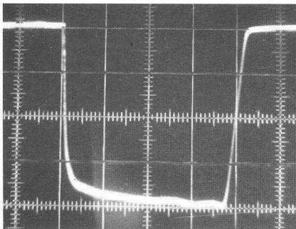
Fig.4.  $\text{H}^-$ -ion source exit beam current. The vertical - 20 mA/div, the horizontal -  $20\mu\text{s}/\text{div}$ .
