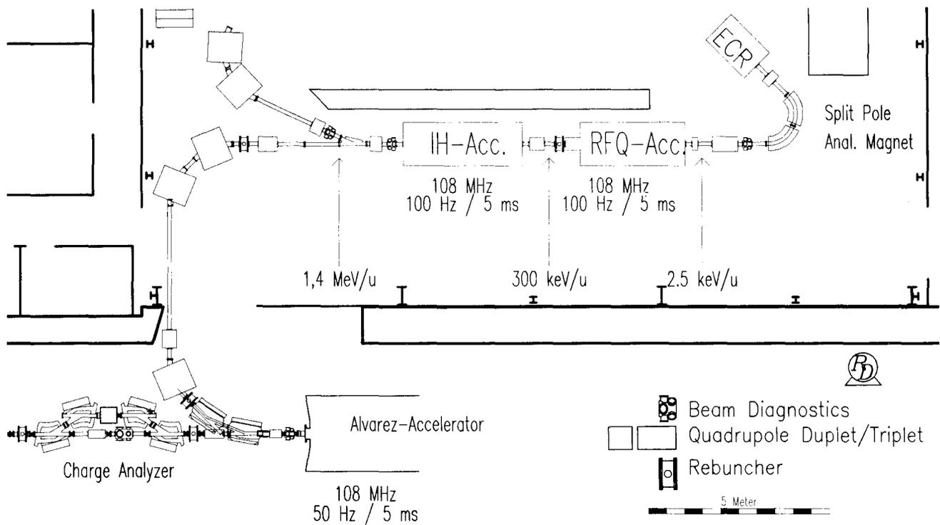
Fig. 4: Schematic of the low-intensity injector
