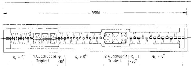
Fig. 6: Schematic view of the IH tank
