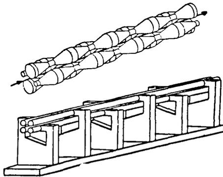
Fig. 5: Schematic drawing of the four-rod RFQ
