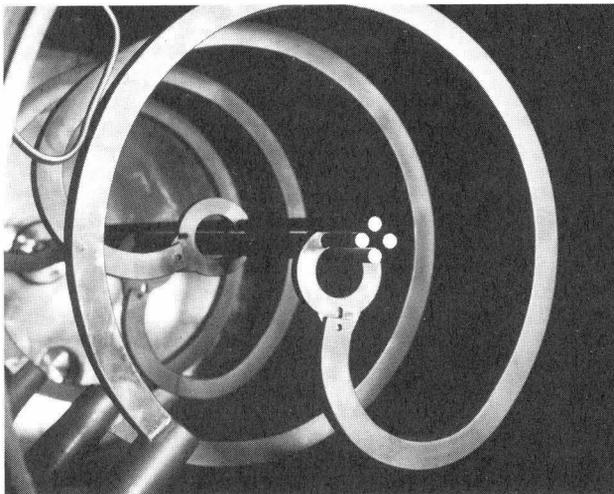
Fig. 7b: Photograph of the spiral resonator
