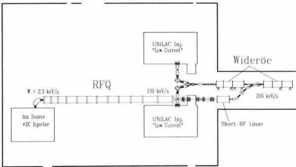
Fig. 2: Layout for injector modification under discussion
