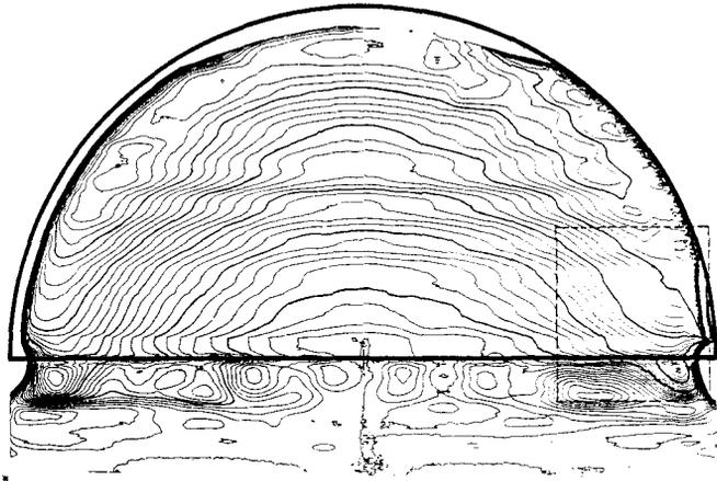
Fig. 10: Field map of the whole magnet at 1.284 T in steps of 2 Gauss each, reference fringe field being subtracted.
