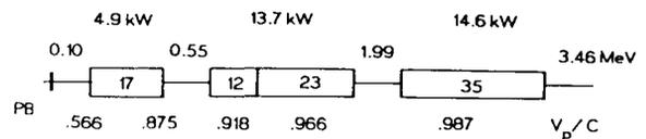
Fig. 6: Scheme of injector linac. PB = prebuncher. Numbers give r.f. power, beam energy, number of accelerating cells and phase velocity respectively.
