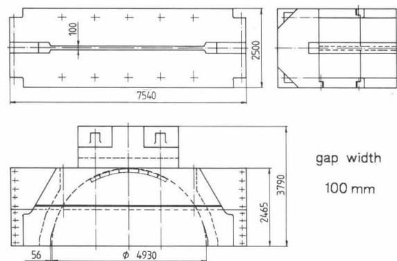
Fig. 9: Construction of the main magnet (reverse field magnet and clamp omitted).
