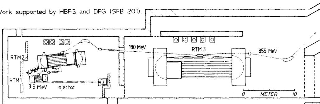
Fig. 2: Plan view of MAMI. First and second RTM stages (left hall) are essentially the ones used for "MAMI A".
