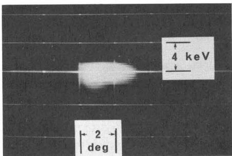
Fig. 7: TV display of the phase space analyser at 100  $\mu$ A beam intensity.
