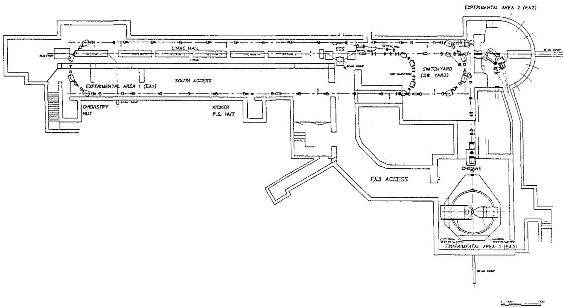
**Figure 1: Pulse stretcher ring layout.**
