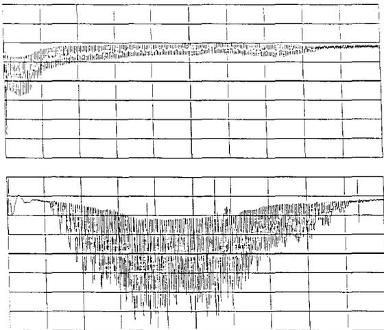
Figure 2: Circulating beam and Extracted beam versus time, 0.5 ms per division.
