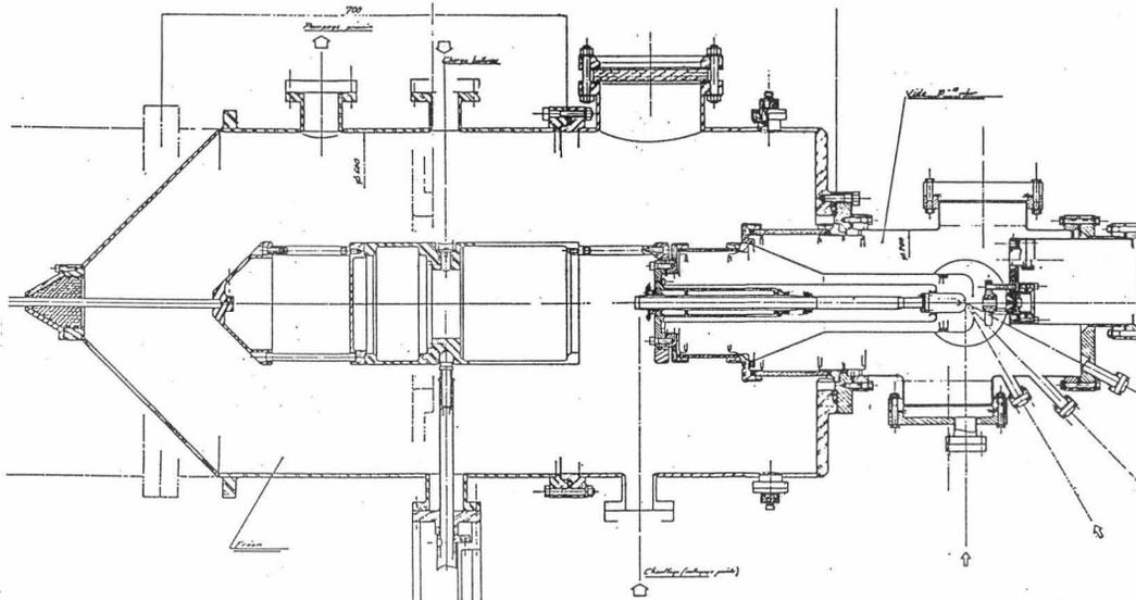
Fig. 6 : General view of the photocathode test bench
