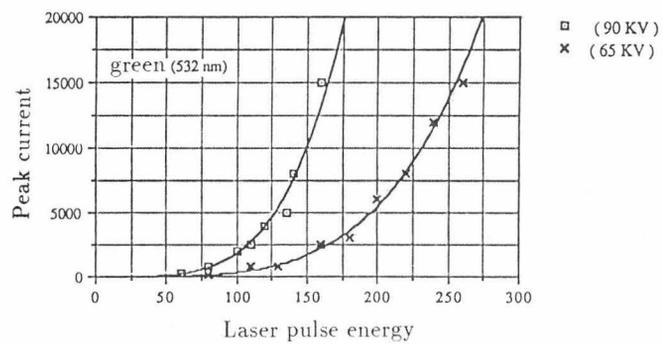
Fig. 10 : Peak current versus laser energy for green light
