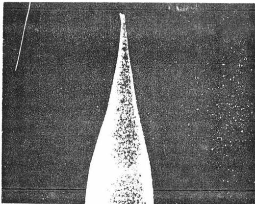
Fig. 7 : Single microscopic W needle (enlarged by a factor  $\approx 400$ )
