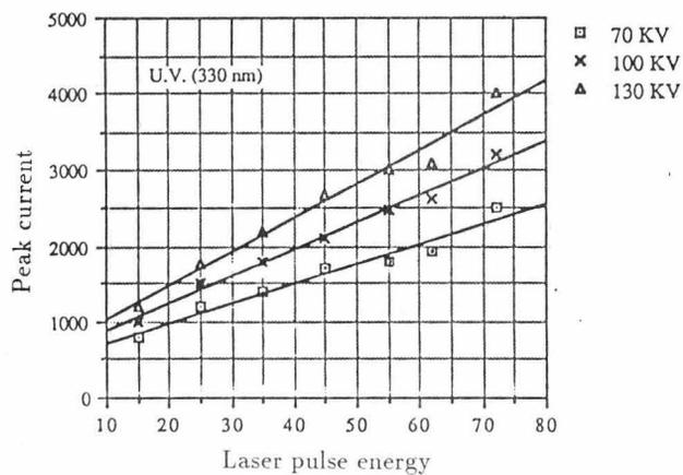
Fig. 9 : Peak current versus laser energy for U.V. light
