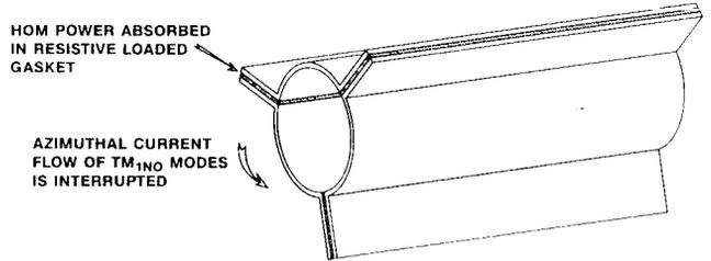
Fig. 4. Advanced cavity design which cannot support azimuthal rf currents.
