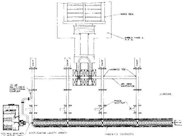
Fig. 1. Schematic of the 200 MeV, 2 kA HCRF Linac. Magnetron driver, phase-locked magnetrons, rf feed, injector, cavities and beam dump represented.
