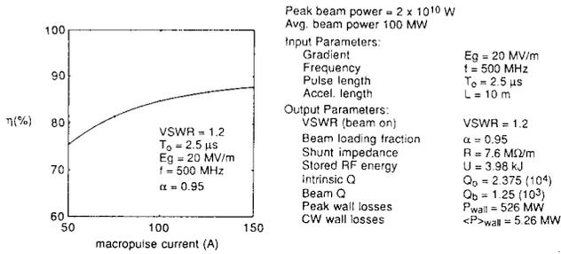
Fig. 3. Results of initial beam loading analysis.
