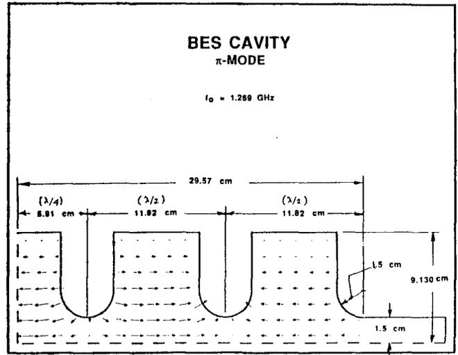
Fig. 2 Electric field distribution in BES cavity.
