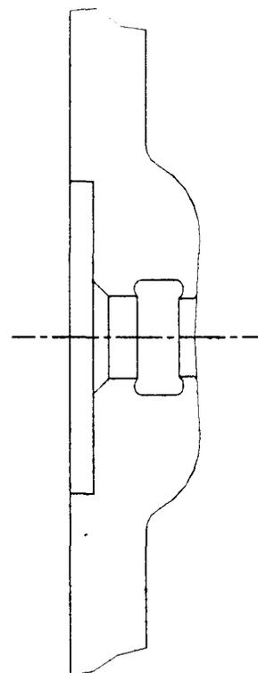
Fig. 2. Enlarged photocathode plug cross section.
