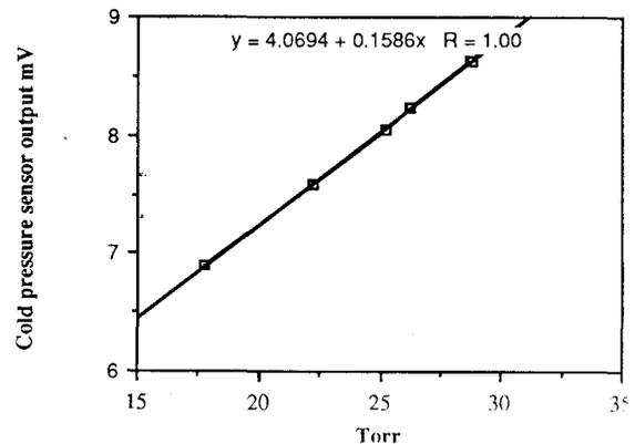
Figure 1. Cold pressure sensor output as a function of pressure at LHe temperature.
