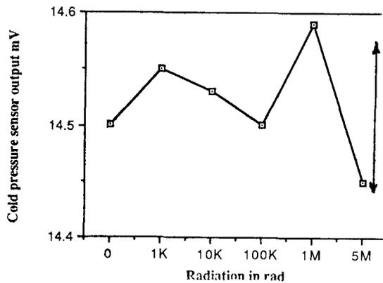
Figure 4. Radiation effect on cold pressure sensor at 4.2K.
