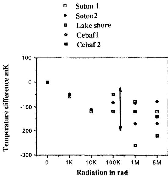
Figure 3. Radiation effect on temperature sensors at 4.2K.
