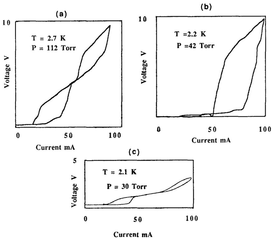
Figure 2 V - I characteristics of LHe level sensor at different temperatures
