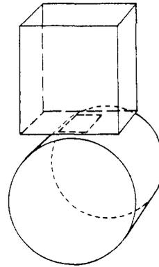
Fig. 1. Diagram of a pillbox cavity coupled to a waveguide.
