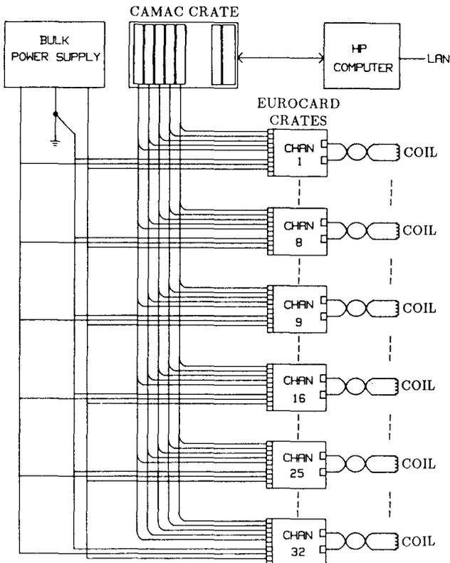
Figure 1 System Block Diagram
