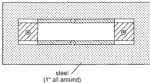
Figure 2. Schematic cross-section of the Panofsky quadrupole.
