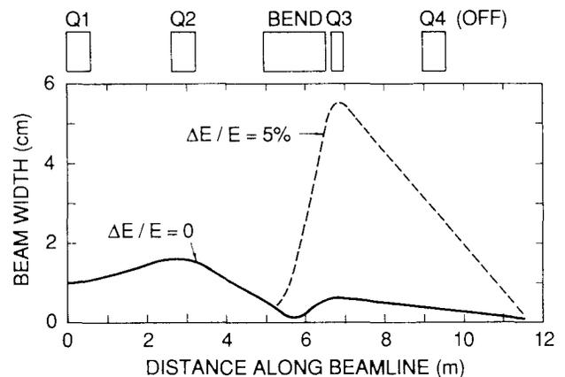
Figure 5. Beam profile for the same beam parameters as Figure 3, but with the spectrometer in the no-resolution mode.
