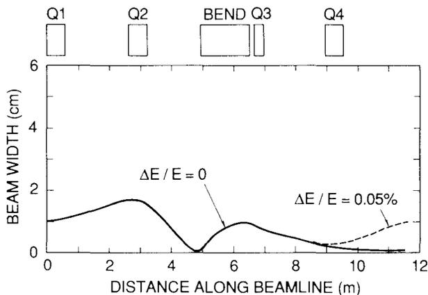
Figure 3. Beam profile (FWHM) for a 100-MeV beam with a normalized emittance of  $20 \pi$  mm-mr, shown for the spectrometer set in the high-resolution mode.
