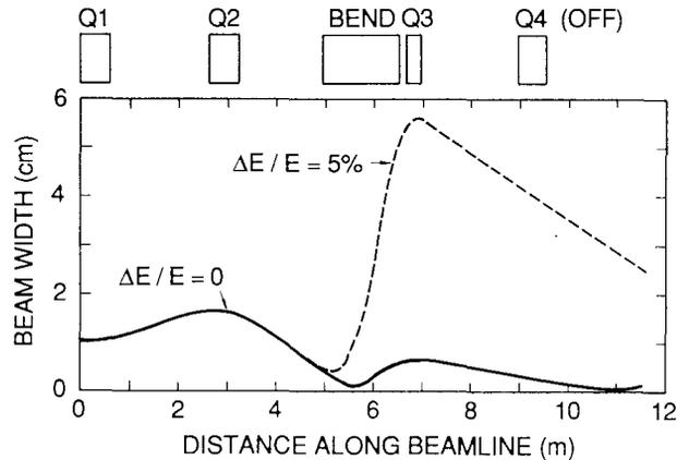
Figure 4. Beam profile for the same beam parameters as Figure 3, but with the spectrometer in the low-resolution mode.
