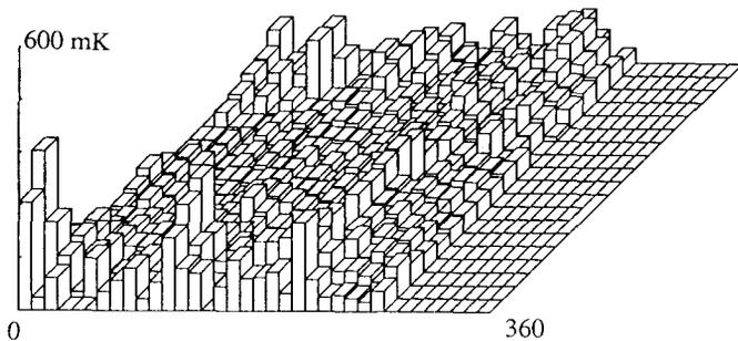
Fig. 4a T-map at a field of 24 MV/m reached after He processing with a CT cavity, showing large number of emitters.
