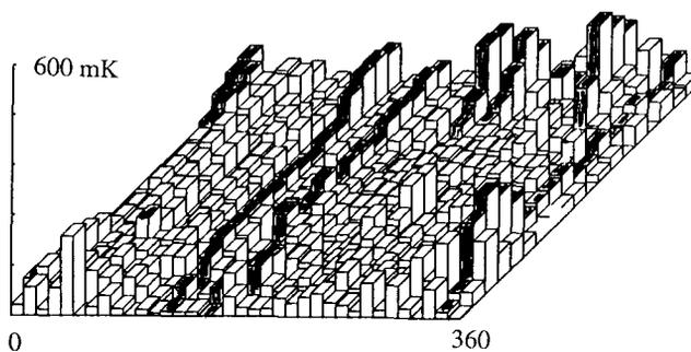
Fig. 5a The highest field T-map ever recorded. Here  $E_{pk}$  was 46 MV/m and  $H_{pk}$  was 1150 Oe. The emission heating areas are shaded. FE is still the dominant problem at this field level, reached after He processing.
