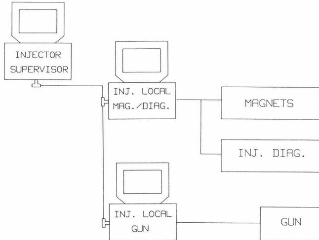
Figure 4 Injector Distributed Architecture
