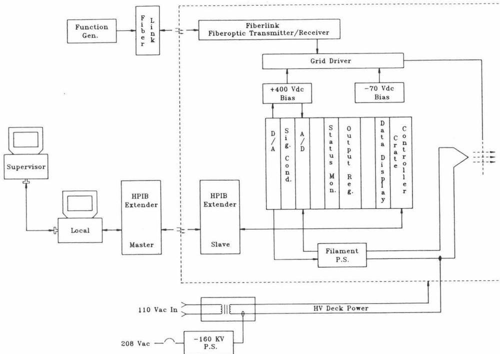
Figure 3 Thermionic Gun Control System Block Diagram
