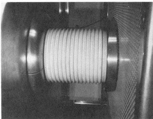
Figure 1 Photograph of the Electron Gun Installed in the High Voltage Deck
