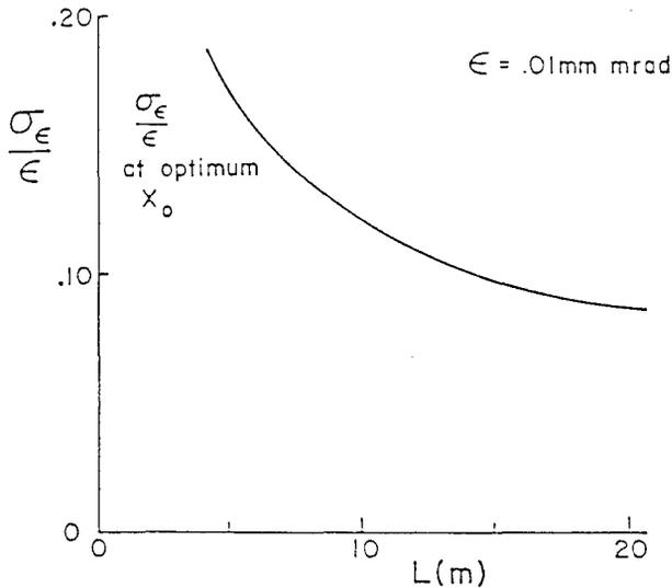
Fig. 4: Precision of emittance measurement  $\sigma_{\epsilon}$  at optimum  $x_0$  and  $z_0$  vs. monitor separation  $L$ , for  $\epsilon = 0.01 \text{ mm} \cdot \text{mrad}$ .
