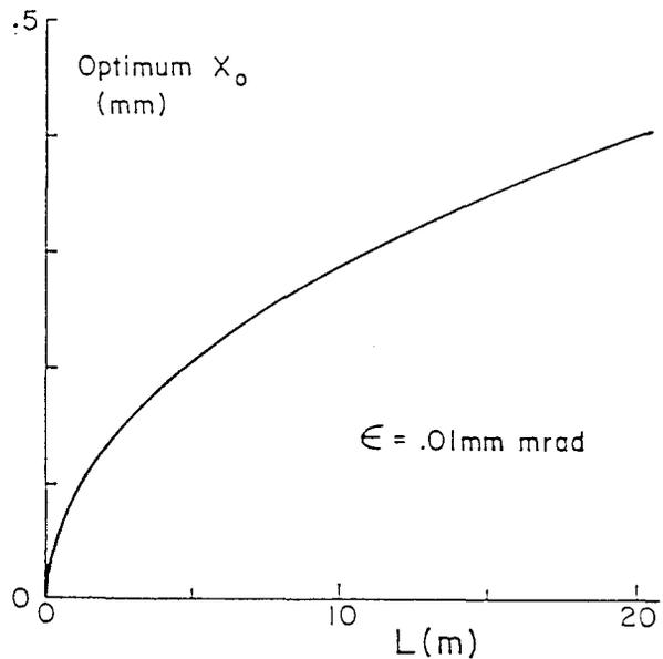
Fig. 3: Waist size  $x_0$  for optimum emittance measurement vs. profile monitor separation  $L$ , for  $\epsilon = 0.01$  mm · mrad.
