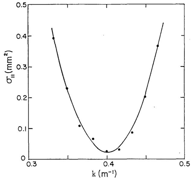
Fig. 5: Square of the horizontal beam size  $\sigma_{11}$  vs. strength  $k$  of a quadrupole singlet  $8.03 \text{ m}$  upstream from the measurement point. The points are experimental data, and the curve is the best fit parabola.
