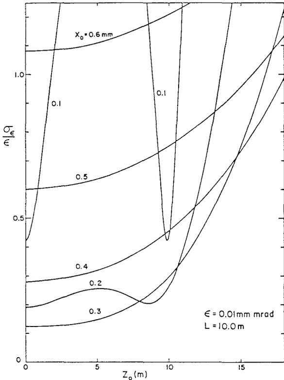
Fig. 1: Precision of emittance measurement  $\sigma_\epsilon$  vs. location of waist  $z_0$ , for different waist sizes  $x_0$ . Here  $L = 10$  m and  $\epsilon = 0.01$  mm · mrad.
