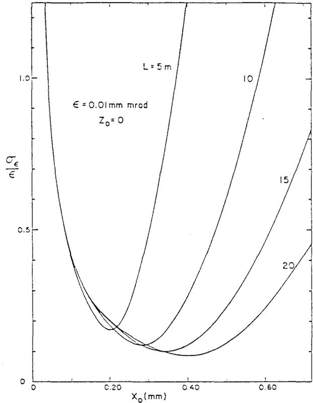
Fig. 2: Precision of emittance measurement  $\sigma_\epsilon$  vs. waist size  $x_0$ , for different profile monitor separations  $L$ . The waist is located at the center monitor ( $z_0 = 0$ ), and  $\epsilon = 0.01$  mm · mrad.
