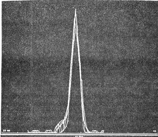
Fig. 4: Accumulation of many beam profile measurements.
