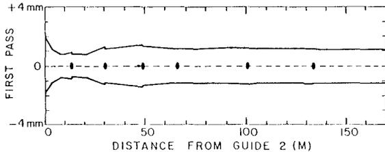
Fig. 1: Computer Simulation of beam envelope using a "weak focussing" solution. Ellipses on axis represent location of quadrupoles.
