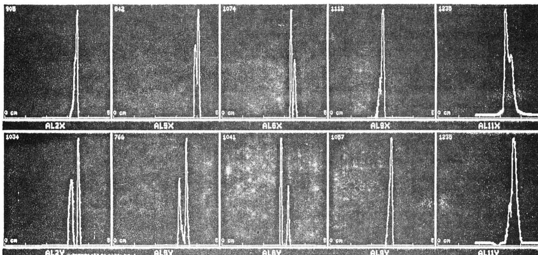
Fig. 5: Beam profile Measurement with two beams in accelerator .
