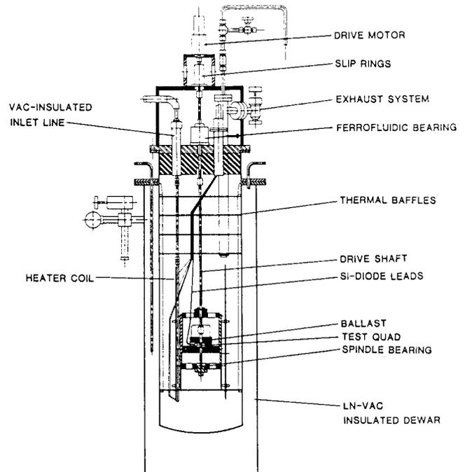
Fig. 3. Cryogenic test Dewar for full quadrupole testing at 20 K.
