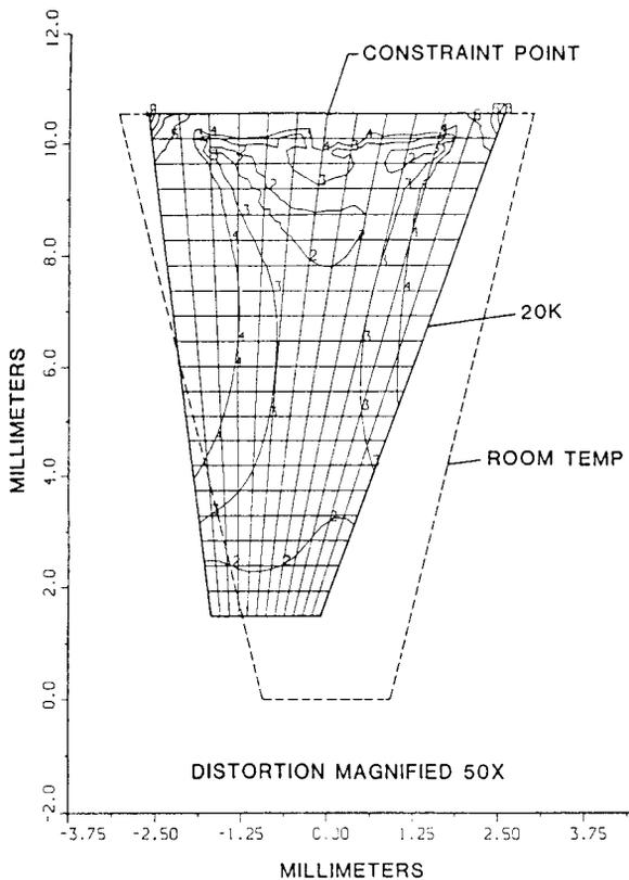
Fig. 2. Thermal distortion of Sm-Co quadrupole segment caused by difference in expansion coefficients.
