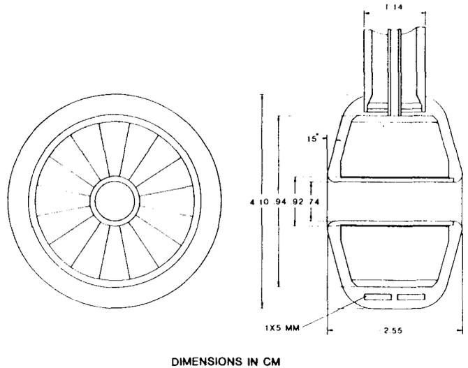
Fig. 1. Small-sized drift tubes and quadrupoles required at 850 MHz.
