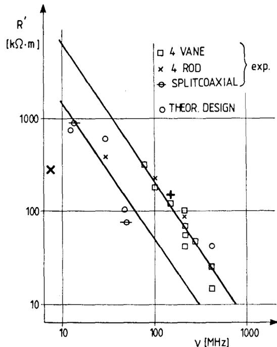
Fig.3 RFQ Impedance as function of frequency
