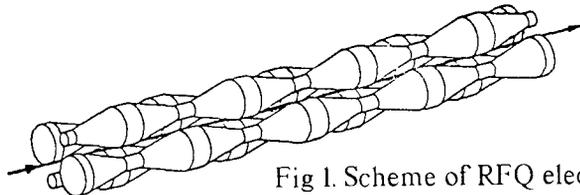
Fig 1. Scheme of RFQ electrodes
