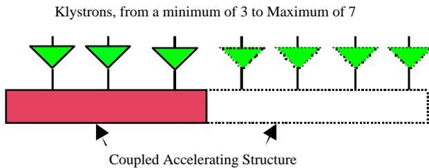
Figure 2: A Block Diagram of a supermodule showing the size variation. Each supermodule has one more klystron than is needed for full-current operation.
