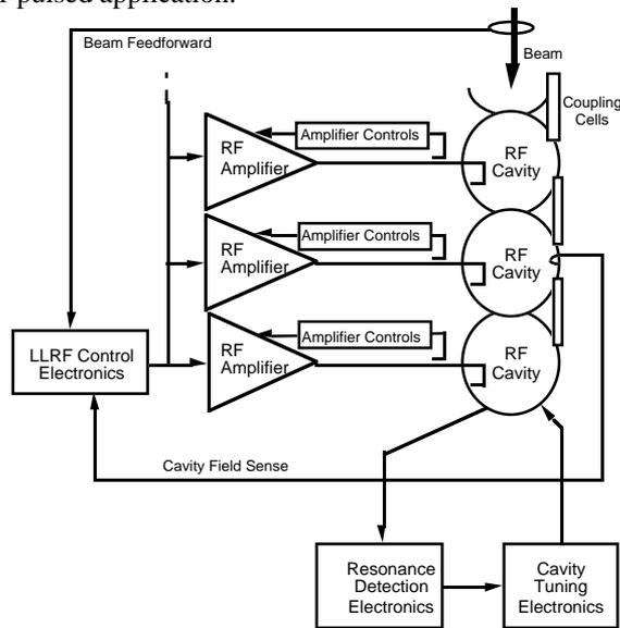
Figure 4: LLRF control diagram for a supermodule. The long coupled accelerator structure is driven by multiple klystrons and controlled with one feedback system. To equalize the klystrons, each one has a control loop.
