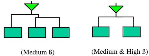
Figure 3: Block diagram of RF system for the superconducting cavities. Each klystron drives either 2 or 3 cavities. The medium and high  $\beta$  refer to the two types of superconducting structures used in APT. [1]
