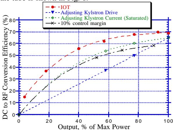
Figure 7: Comparison of the operating efficiency characteristics of the HOM-IOT and a standard klystron.
