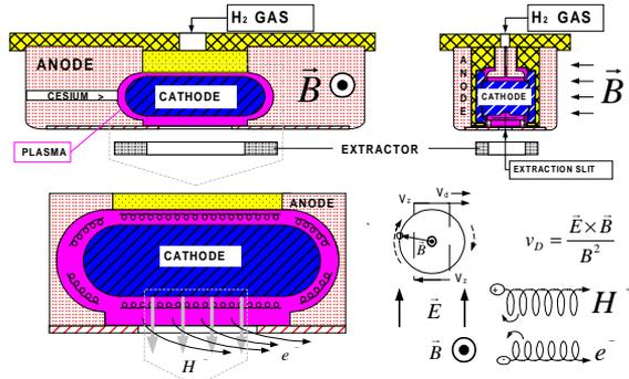
Figure 2: Magnetron source and  $E \times B$  drift.
