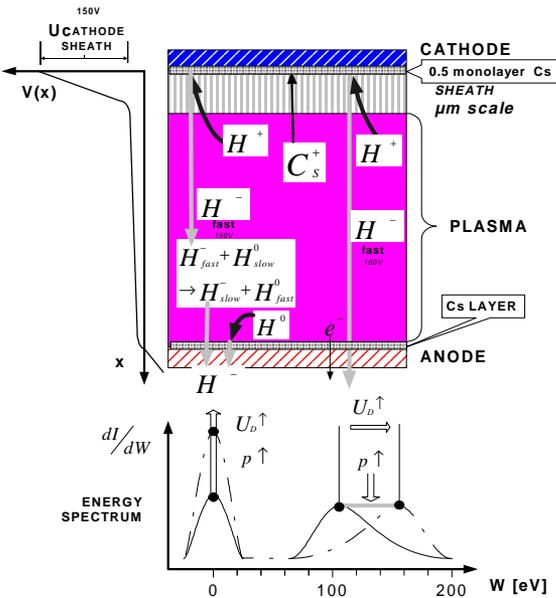
Figure 3: Production of  $H^-$  at cathode and anode of the source and their energy spectrum.
