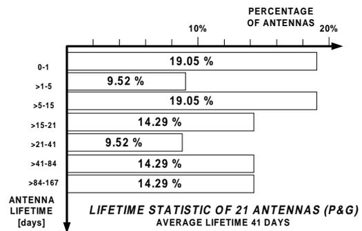
Figure 10: Lifetime statistic of the coated antennae.
