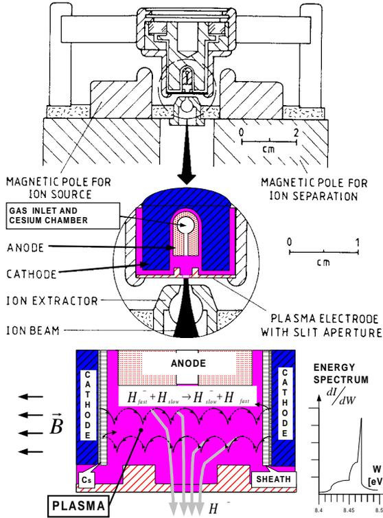
Figure 5: Penning source schematic and its energy spectrum.
