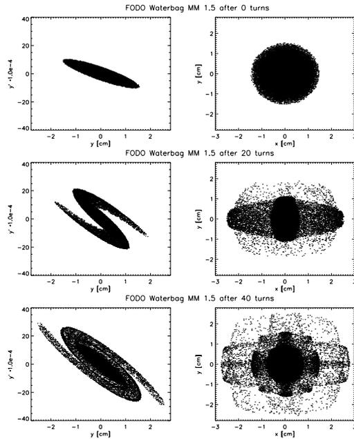
Figure 7: 2d-simulation (particle-in-cell) of halo development for a coasting beam in a FODO synchrotron lattice with weak space charge and 50% mismatch (shown are  $y$ - $y'$  and  $x$ - $y$  projections after 0,20,40 turns).
