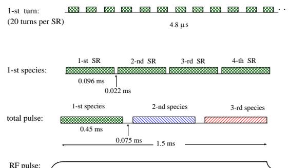
Figure 3: Linac pulse structure.
