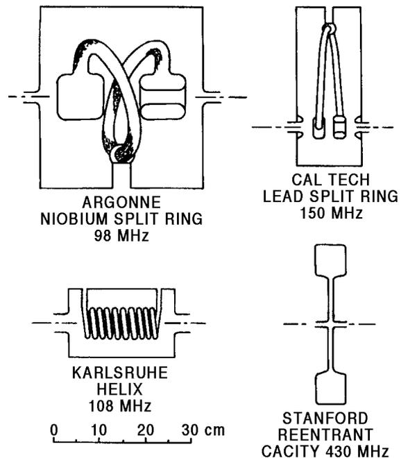
Figure 1: Heavy-ion accelerating structures in 1977.
