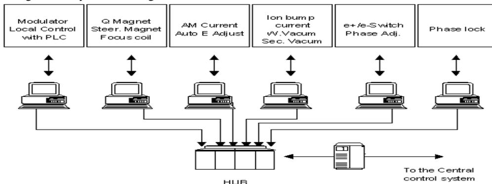
Figure 2: Linac Control System
