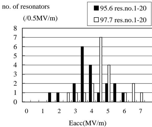
Fig.2 Histograms of the field gradients at rf input of 4 watts of the first 20 resonators measured in June, 1995 after normal all-together precooling mode and July, 1997 after three-by-three module sequential mode.
