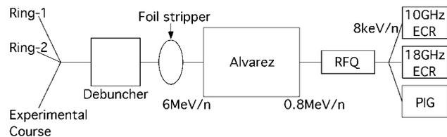
Fig.1 Schematic drawing of the HIMAC injector. Under TSA operation, one injector works as if it were three.
