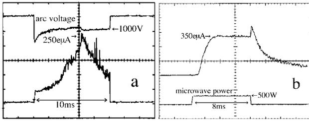
Fig.3 Pulsed beam-waveforms for PIG (a) and 10GHz-ECR (b). In such a low-duty pulsed PIG, the output of  $\text{Ar}^{8+}$  (highly-charged ions) is high during the early 6-7ms [4]. For the production of  $\text{C}^{6+}$  in the 10GHz-ECR, a smooth and rapid rising, and a clear afterglow-peak seem to be essential as an indication of stable operation.
