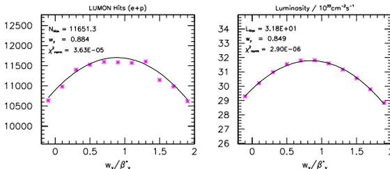
Figure 2: Scan of the vertical waist. Parabolic fits are drawn through the data points
